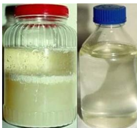
Figure 1. Coconut Milk Fermented by Probiotic Starter Culture after Incubation at Room Temperature (A); and the Obtained FCO after Filtration using Whatman Filter Paper (B).
