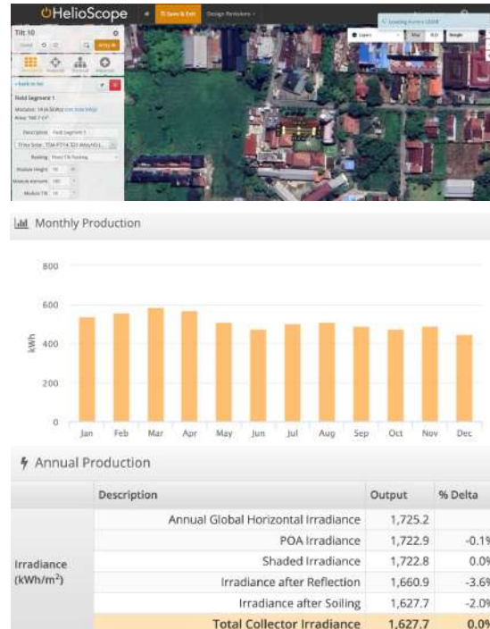
Figure 2. HelioScope Process and Result: (a) Site Selection, (b) Monthly Production, (c) Annual Irradiance Source: HelioScope, 2025
