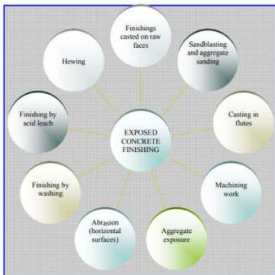
Gambar 2. Prosedur Finishing Semen Ekspos Sumber: Tudora, 2011
